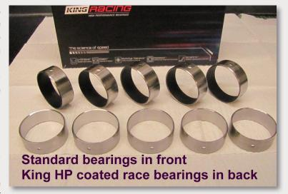
RPMs climb the demands also increase. Choosing the right bearing includes its structural integrity, intermediate layering, bearing overlay material, adhesion qualities, oil grooving, oil hole placement, eccentricity/concentricity, crush and wall thickness variations. We'll get into these issues a bit deeper in the next issue.
