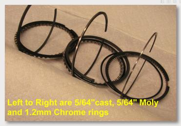
efficiently. The rings aren't relied upon as heavily but still have the same job and have been reduced to 1.2 to 1.5mm and radial tensions are lower. This reduced heat, helps engine power and should go hundreds of thousands of miles, with proper care, before it needs to be rebuilt.
