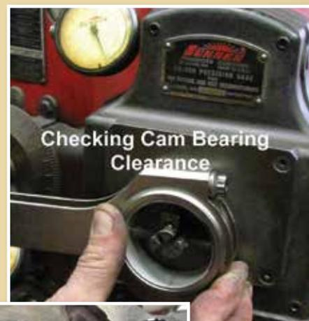
Checking Cam Bearing Clearance
