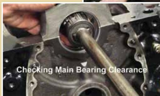
Checking Main Bearing Clearance
