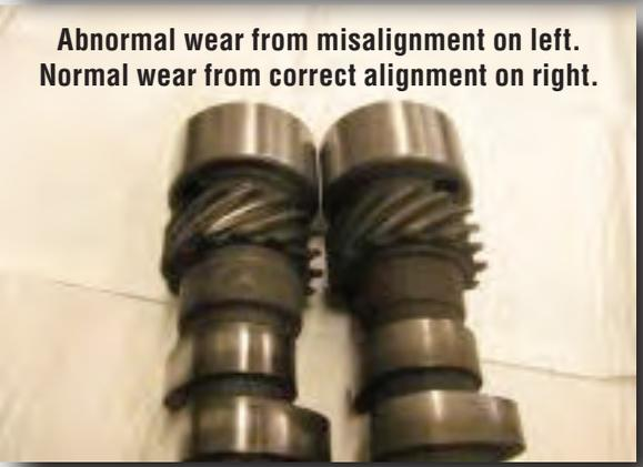
Abnormal wear from misalignment on left. Normal wear from correct alignment on right.
