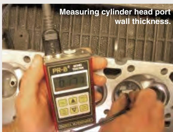
Measuring cylinder head port wall thickness.
