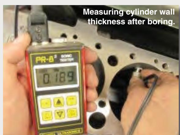
Measuring cylinder wall thickness after boring.
